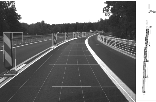
Fig. 12. Highway scenario: construction area - driving area delimiters (poles and fences) successfully detected and tracked.
